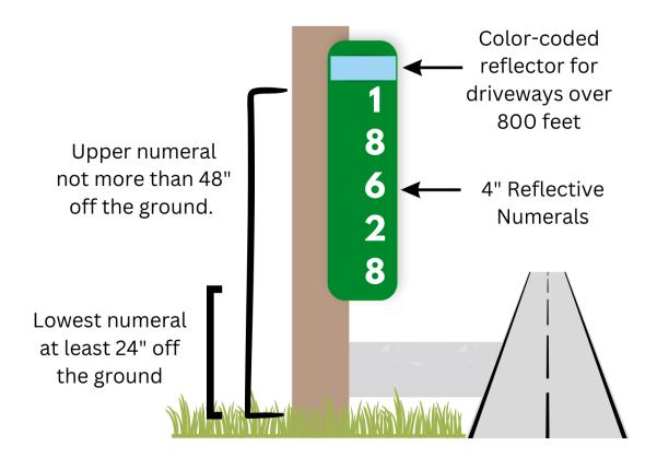
The post shall be located not more than 20 feet from the road right-of-way and not more than 10 feet from the vehicular entrance or drive to the principal building.
